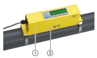
➤ Set the electronics module (1) on the guide rail (2) and engage it in the clamp connections at both ends.
