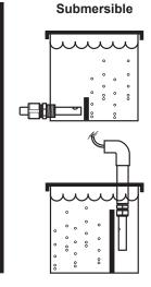
Use caution to avoid air bubbles or sediment trapping inside the electrode cavity.
